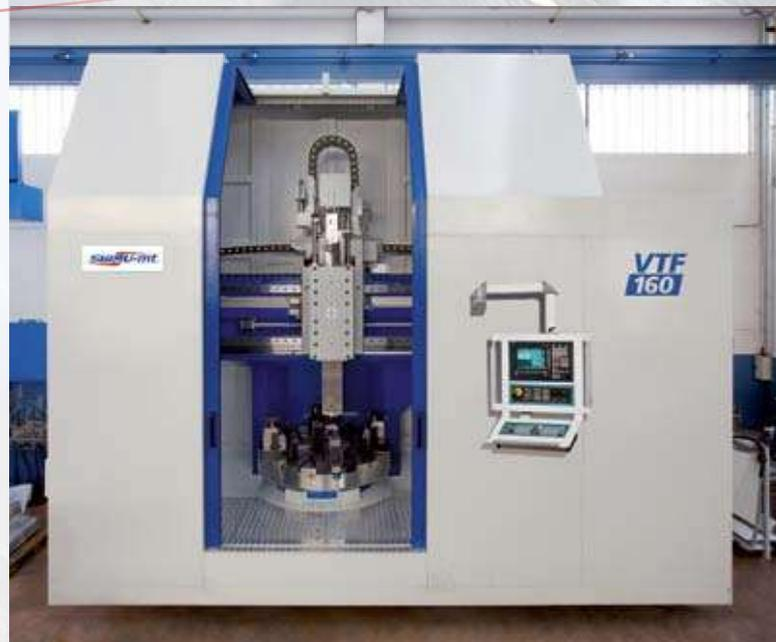
**complete railway wheel machining.**
